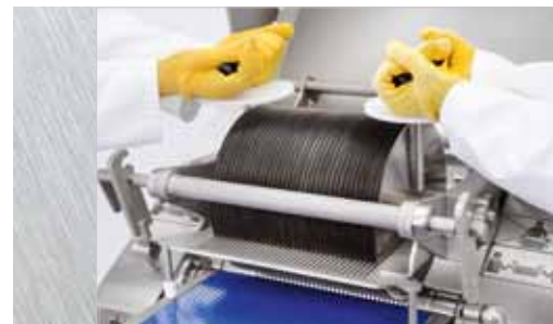
ESB 4434 SH: Removal of cutting roller
